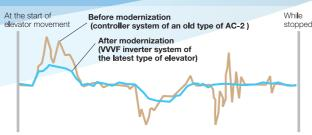
"VVVF inverter method: Simultaneously controls voltage and frequency and employs the right amount of torque control. This controller method consistently maintains noting a movement of elevators.
