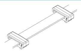
1) Where additional mechanical strength is required, e.g snow, strong winds etc, the spacing between the fasteners should be ≤300 mm.
