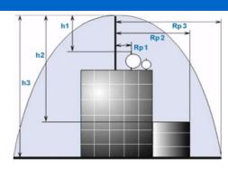
NP: Level of protection calculated as per ANNEX B of NFC 17-102 standard.
