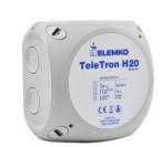
protection against inducted surges (8/20µs) generated by the electromagnetic field, which is created by a nearby lightning strike. The surge protective devices are generally placed at each end of the line and as possible as close to the device to be protected. It is providing protection between the pair and earth (common mode) and also between the poles of the pair (differential mode).
